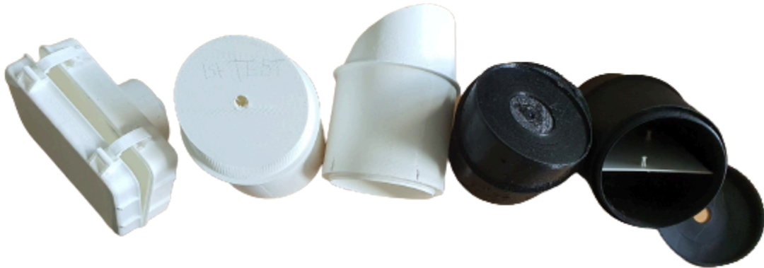
Figure 3: Selected iterations of the designed case for WaziSenseV2.
