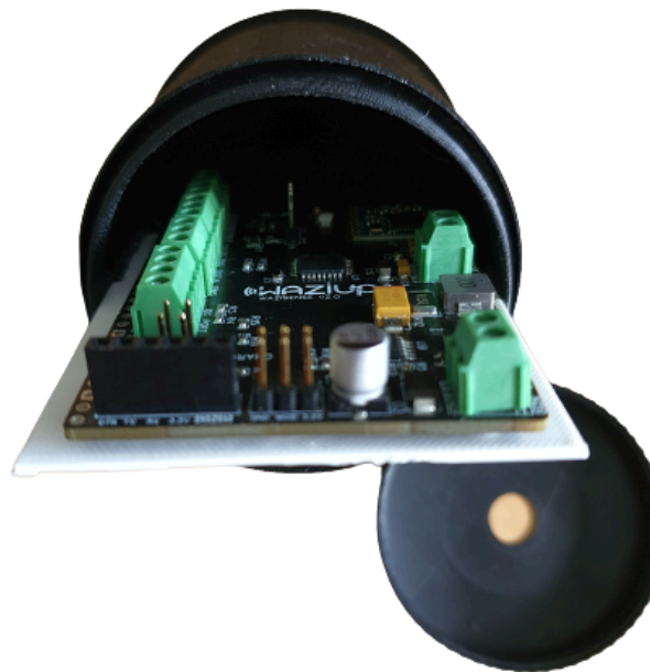
Figure 4: Last iteration from below with opened service cover, for easy access.
